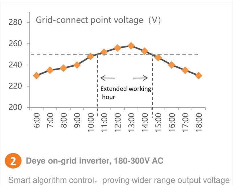
to reduce inverter stop working due to high AC voltage
